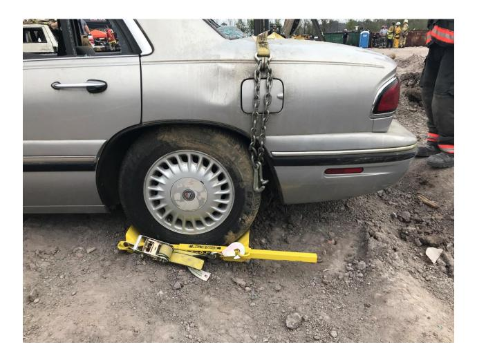
These issues were cleared with the latest model. We now have a lightweight wheel chock with a means to capture a wheel within the wedges and a means to drive pickets through the device and into the ground. Concerns of a passenger car rolling or sliding are virtually eliminated with the Res-Q-Jack Ratcheting Wheel Chock otherwise known as the "Ratchock" or "WheeLock".
