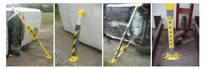
Pictured above are FRP (fiberglass reinforced polymer) composite prototypes from Res-Q-Jack. Due to poor testing results Res-Q-Jack concluded that this material has no place in the extrication environment.
