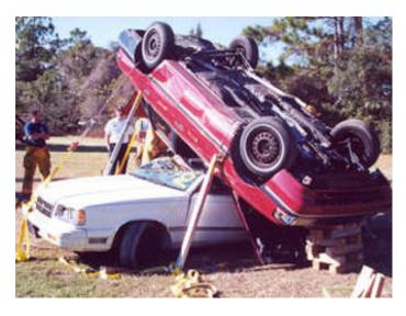
A vehicle completely out of contact with the ground requires a reasonable amount of attention. This team chose to stabilize the front of the upper vehicle with 1 box crib, 2 Res-Q-Jack® adjustable stands and a chain saddle.
