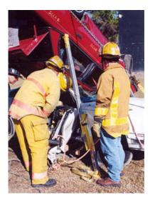
The Jack Stands permitted the crew to gently lift the rear of the upper vehicle off the passenger side of the lower vehicle's roof.
