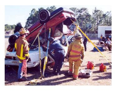
The rear of the vehicle is stabilized with 2 Res-Q-Jack® Jack Stands, 3 tie lines, and 1 picket. The tie line attached to the picket is meant to keep the vehicle from moving forward.
