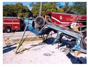
With vehicle properly stabilized, the roof may be removed as shown above at Broward County (FL). A stake in the hood and the tie line at the rear restrict forward and rearward vehicle movement.
