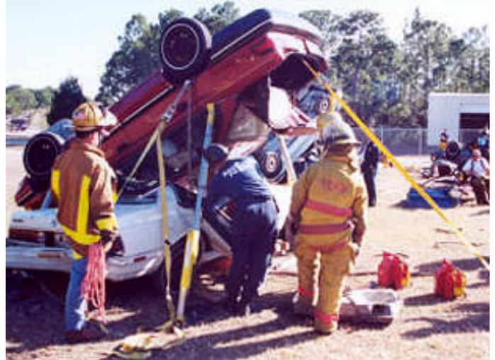
The rear of the vehicle is stabilized with 2 Res-Q-Jack® Jack Stands, 3 tie lines, and 1 picket. The tie line attached to the picket is meant to keep the vehicle from moving forward.
