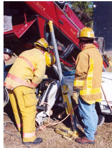
The Jack Stands permitted the crew to gently lift the rear of the upper vehicle off the passenger side of the lower vehicle's roof.
