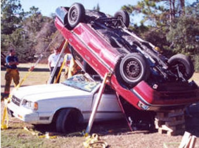
A vehicle completely out of contact with the ground requires a reasonable amount of attention. This team chose to stabilize the front of the upper vehicle with 1 box crib, 2 Res-Q-Jack® adjustable stands and a chain saddle.
