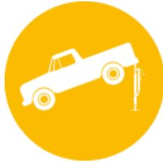
The Aluminum X-Strut® – fully assembled with head and pivoting base and fully extended to a maximum height of 98 inches – is safe to 9,700 pounds in the center (it didn't fail in testing until almost 20,000 pounds), 6,700 pounds at the tip of the round point (failed at 13,400 pounds), and 5,600 at the tip of the chain grab (failed at 11,200 pounds).
