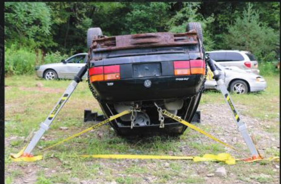
D ROOF-RESTING REAR LIFT
