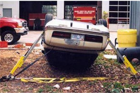
Basic or initial roof resting stabilization performed at Orange County (FL) Fire Dept. Note the straps extending from base up to trunk lid. These straps will help restrain sway
