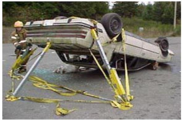
Additional stability can be applied by adding a third stand at the rear as shown here in Dupont, WA. Note the counteracting directions of the straps.
