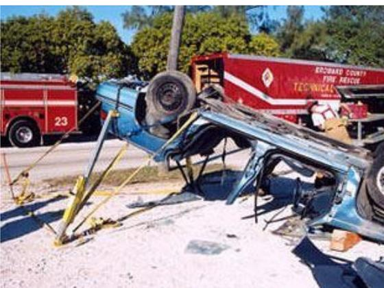
With vehicle properly stabilized, the roof may be removed as shown above at Broward County (FL). A stake in the hood and the tie line at the rear restrict forward and rearward vehicle movement.
