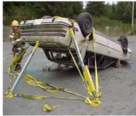
Additional stability can be applied by adding a third stand at the rear as shown here in Dupont, WA. Note the counteracting directions of the straps.
