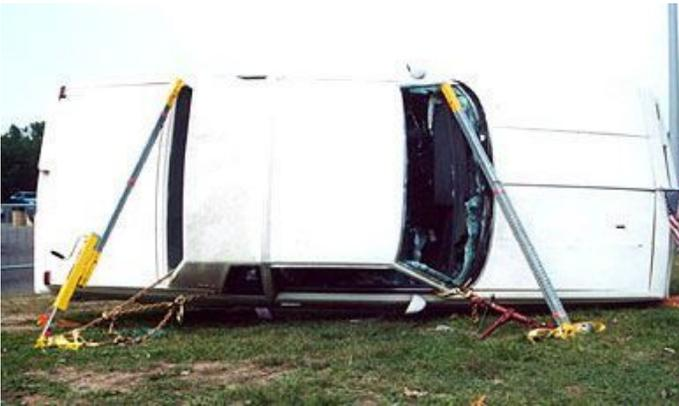
This setup illustrates the placement of the jack stands across from each other and the adjustable stands across from each other on opposite sides of the vehicle. Naturally, the jack stands would be at the end of the vehicle to be lifted.
