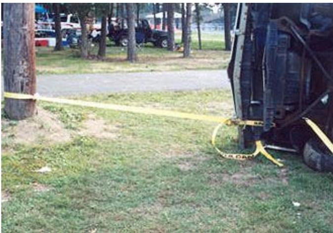
This picture shows the vehicle tied to a pole up hill and in front of the vehicle to restrain front to rear movement of the vehicle.
